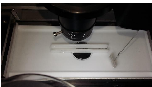
Figure 14 : a) The ISR can be combined with a KSV NIMA Langmuir trough. This figure depicts our set up. b) Schematic representation of the magnetic rod interfacial stress rheometer. This image has been taken from BROOKS ET AL. (1999)
