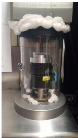
Figure 5.2. Photo of the solvent trap setup (first approach), where in the peltier sample is placed and it is sandwiched with the upper cone-plate. A metal ring is attached to the peltier and in the top of the ring there is a plastic cover. The outer part is a big plastic cover which isolates the sample from the external environment. Cottons in the top (dry) placed in order to improve the isolation and in the bottom (wet) in order to keep the concentration constant.
