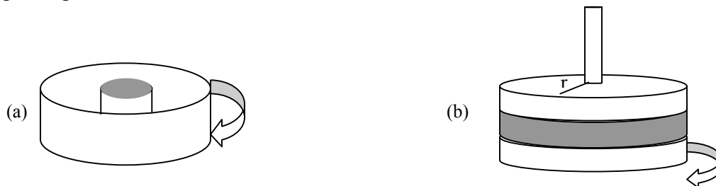
Figure 2.7 Schematic representation of (a) the Couette and (b) parallel plate geometry
