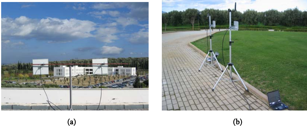
Figure 3.11: The testbed setup for the outdoors experiments (a) with 27dBi patch panel antennas on the post, (b) with 19dBi patch panel antennas on tripods.
